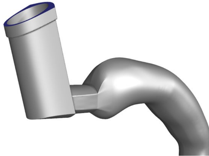
Computer aided design model of fluticasone propionate inhalation metered aerosol and mouth-throat model – internal FDA model.
