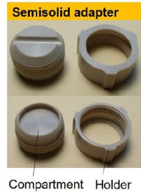
C: USP apparatus 4 with semisolid adapters
