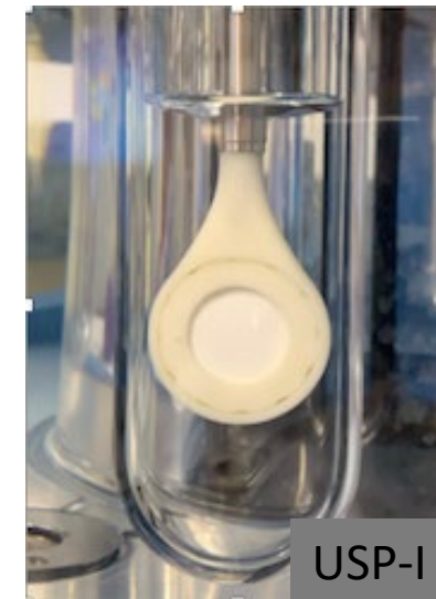
3D-Printed Two-side Adapter in USP apparatus I
