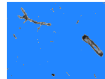
Threshold = 175 Aim for a thin gray border around the edge of the particles and a complete perimeter.
