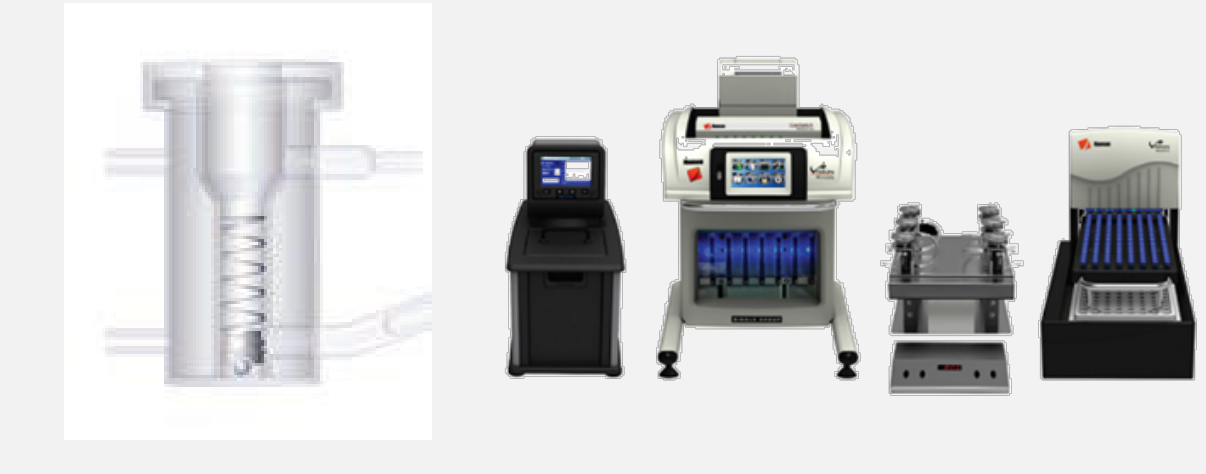
Figure 2: Images of (left) Vision Microette vertical diffusion cell and (right) Vision Microette test system
