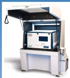
Icon-IR AFM-IR instrument (Bruker, Santa Barbara, CA, USA) used for analysis.
