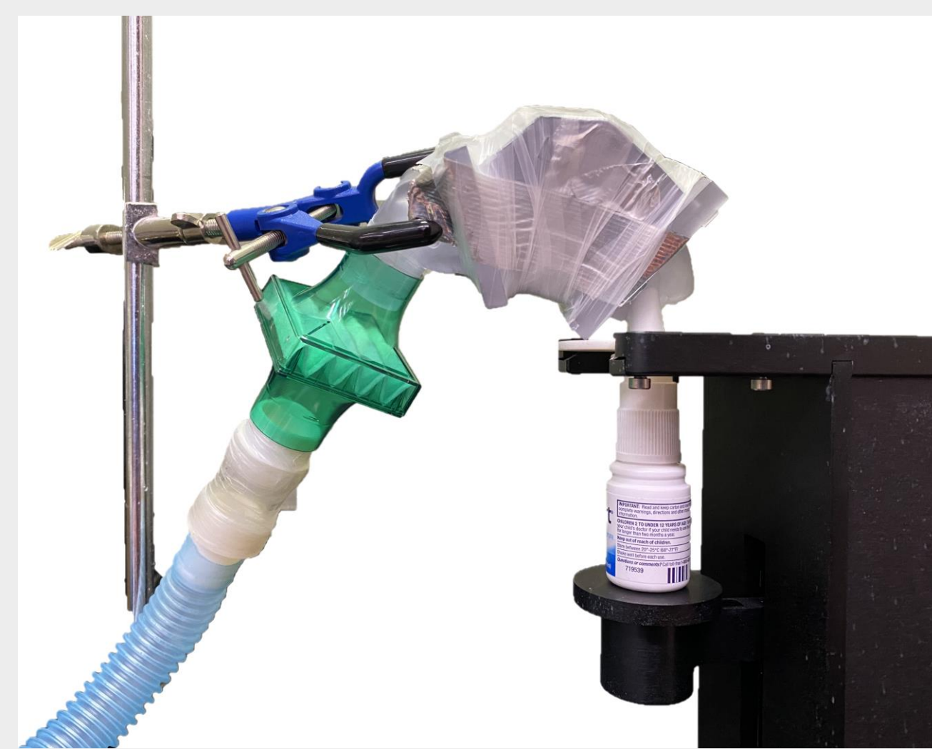
Figure 4 – Experimental setup of the controlled administration method. The nasopharynx component is connected to a filter, which is connected to a breathing machine via blue ventilator tubing.
