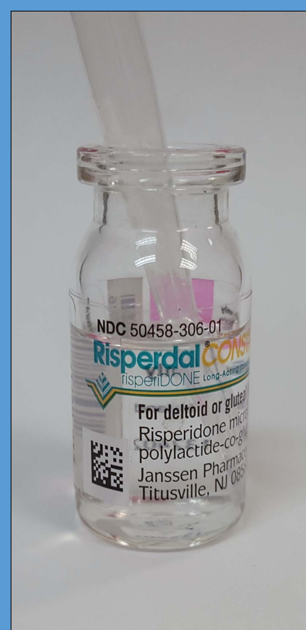
Fig. 1. Dissolution of PLGA microparticles with DCM.
