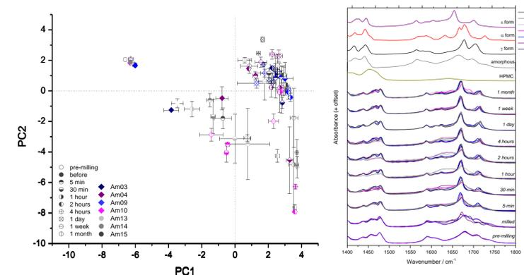
Figure 4. Simplified PCA analysis results of the ATR-IR spectra collected from the samples which were milled for one cycles at various time points. (a) Scores plot of spectra (mean ± sd, n=3) and (b) the associated representative spectra of these samples with reference indomethacin polymorph spectra.
