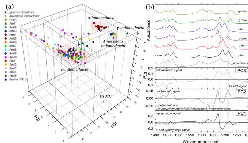
Figure 2. PCA analysis of the ATR-IR spectra collected from the samples at various time points. (a) Scores plot of the first three principal components (PCs) and (b) the associated loadings for these PCs with IR spectra of the indomethacin polymorphs for comparison.
