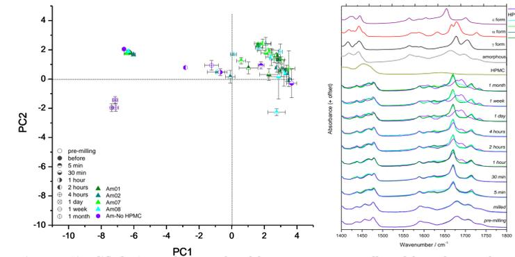
Figure 3. Simplified PCA analysis results of the ATR-IR spectra collected from the samples which were not milled at various time points. (a) Scores plot of spectra (mean ± sd, n=3) and (b) the associated representative spectra of these samples with reference indomethacin polymorph spectra for comparison.
