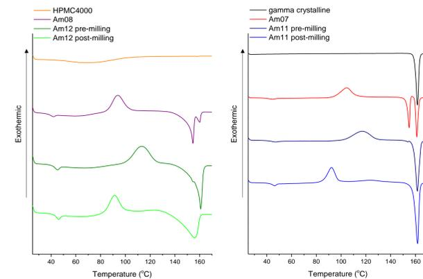
Figure 1. DSC thermograms of representative samples of the amorphous indomethacin before and after dry milling before addition to the suspension vehicle.
