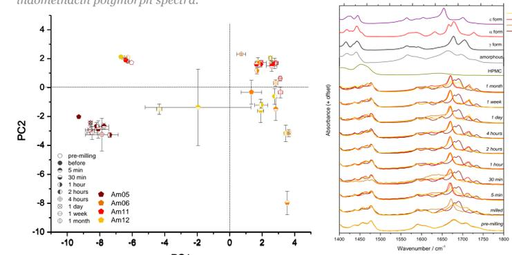
Figure 5. Simplified PCA analysis results of the ATR-IR spectra collected from the samples which were milled for 5 cycles at various time points. (a) Scores plot of the first two principal components (PCs) and (b) the associated representative spectra of these samples with reference indomethacin polymorph spectra for comparison.
