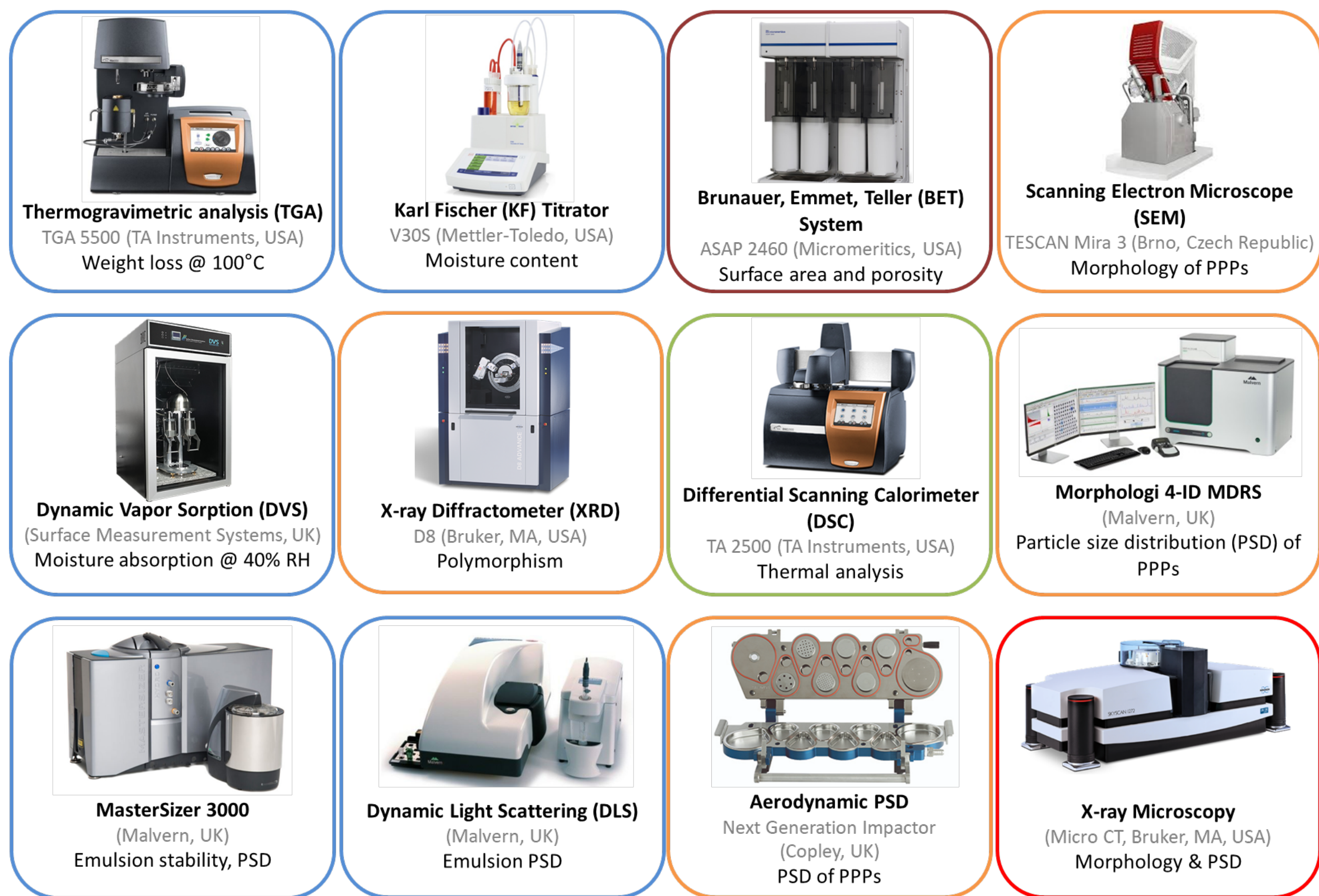
Figure 2. Characterization methods for model drug products.
