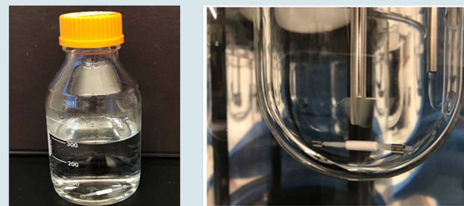
Figure 2. Pictorial demonstration of in vitro drug release from LNG-IUSs using water bath shaker and USP apparatus 2 methods.
